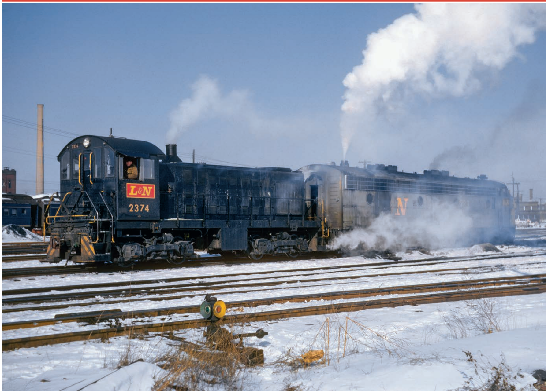
Alco S2 (L&N class S80) 2374 is hostling E7 783 to South Louisville for attention on a very cold and snowy January 30, 1966. The E-unit was purchased secondhand from the Frisco in 1965. The addition of the grill along the top of the car body gave it an E8 look, but internally it was still an E7. On the Frisco, it was 2002, and named for the racehorse "Comanche." —Tom Smart photo
