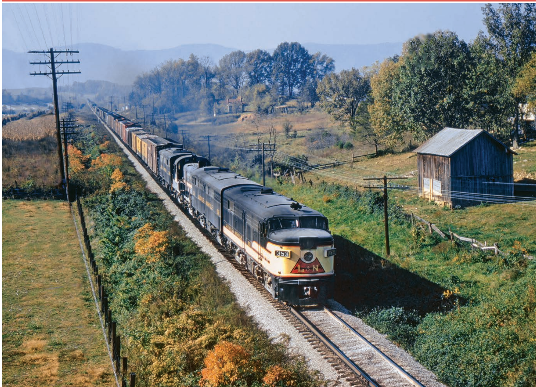
The photographer was on the US 25 overhead bridge at Jacksboro, Tenn. as a northbound Knoxville & Atlanta Division freight came roaring through behind a quartet of Alco motive power. At the time, the stretch between Etowah and Corbin required lead units with ATC (Automatic Train Control). This kept ATC-equipped units captive to the K&A until the system was discontinued in June 1964. — David Salter photo
